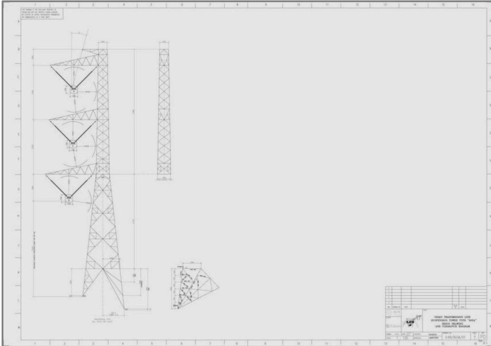
Figure 5: Proposed transmission line suspension tower
